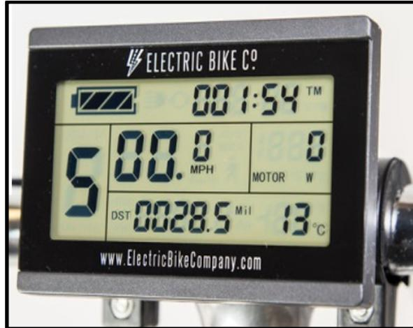
**Note:** It is always safest to mount the bike before turning on the display screen, as turning on the display screen enables the throttle. If you get on and off the bike with the display on, you could accidentally hit the throttle and send the bike forward. If this occurs, you will have better control of the bike if you are straddling the bike and holding onto the handle bars.
